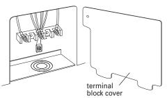
**9** Depending on your electrical supply, make the four-wire or three-wire connection to the range following the "Power supply cord method" or "Direct wire method" instructions for copper wire or aluminum wire depending on the connection needed.
